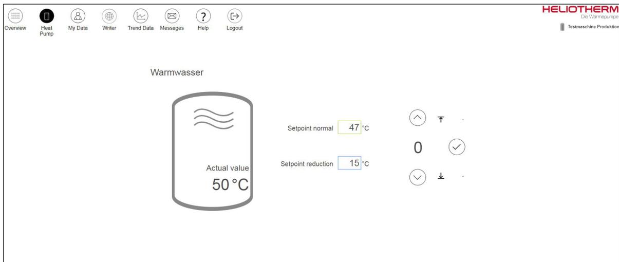
Fig. 9: Submenupoint „Hot Water“ Remote Control Gateway
