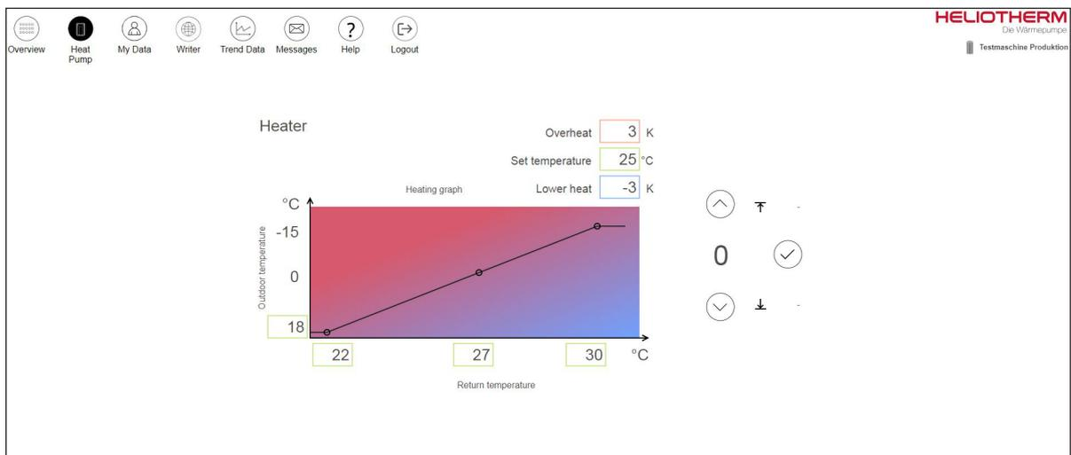
Fig. 7: Submenupoint „Heater“ Remote Control Gateway
