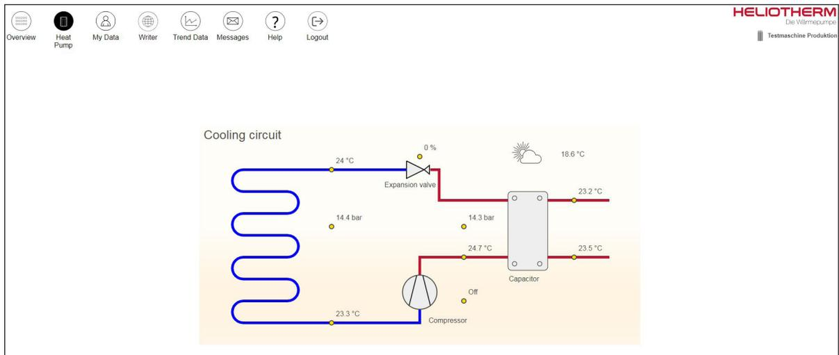
Fig. 11: Submenupoint „Cooling circuit“ Remote Control Gateway
