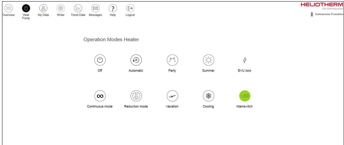
Fig. 5: Submenupoint „Operating Modes Heater“ Remote Control Gateway
